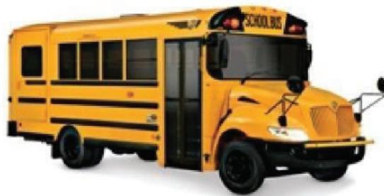
**Type C:** A Type “C” school bus is constructed utilizing a chassis with a hood and front fender assembly. The entrance door is behind the front wheels; also known as a *conventional school bus*. This type also includes cutaway truck chassis or truck chassis with cab with or without a left side door and a GVWR greater than 21,500 pounds.
