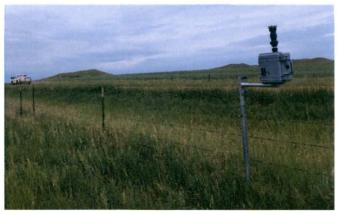
Figure 3. MiniVol<sup>TM</sup> Portable Air Sampler in operation at site #1 (vertically mounted)
