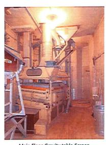
Main Floor-Gravity table-Screen separator-Note duct tape on legs
