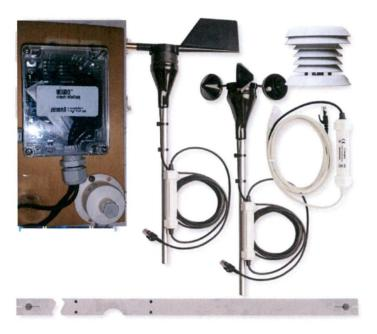
Figure 5. Onset Hobo Data Logger (H21-002) (Image partially from Onset Website www.onsetcomp.com)
